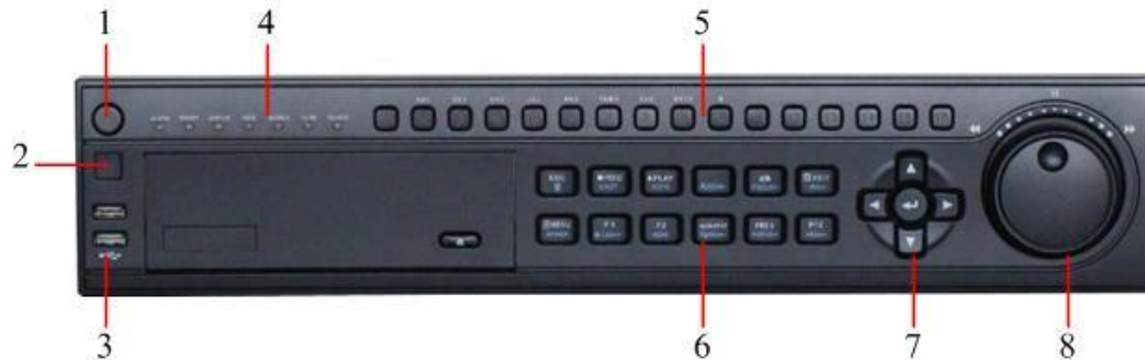
Figure1. DVR Front Panel Controls
